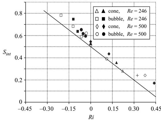
FIGURE 5. Experimental verification of the breakdown criterion. Open and filled symbols correspond to the IC and IH apparatus, respectively. The solid line shows the theoretical criterion.
