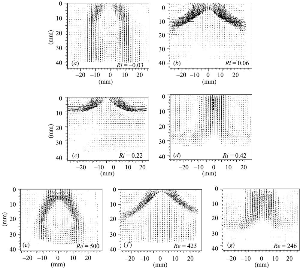
FIGURE 7. Effect of  $Ri$  ( $a-d$ ,  $Re = 246$ ) and  $Re$  ( $e-g$ ,  $\Delta T = 1.1$  K) on the VB configuration at the vertical mid-plane, IC apparatus (jet flows from top to bottom and shown by vector maps averaged over 100 s). ( $a$ )  $S_{int} = 0.64$ , ( $b$ )  $S_{int} = 0.48$ , ( $c$ )  $S_{int} = 0.28$ , ( $d$ )  $S_{int} = 0.13$ , ( $e$ )  $S_{int} = 0.47$ , ( $f$ )  $S_{int} = 0.36$ , ( $g$ )  $S_{int} = 0.15$ .
