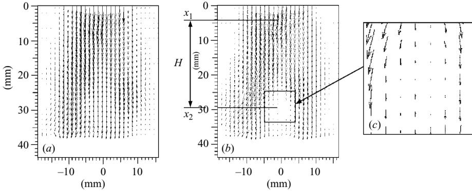
FIGURE 4. Definition of  $H$ . Instantaneous flow field in the vertical mid-plane at critical conditions; jet flows from top to bottom;  $Re = 246$ ,  $Ri = 0$ , and  $S_{int} = 0.53$ . (a)  $t = 0$ , (b) initiation of a stagnation point at  $t = 2$  s, (c) closeup of the stagnation point region.
