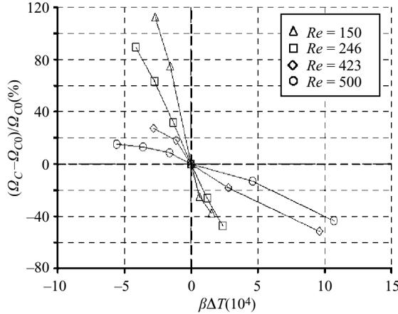
FIGURE 6. Delaying/advancing the onset of vortex breakdown by thermal effects in the range  $150 \leq Re \leq 500$ , IC apparatus.  $\Omega_{C0} \equiv \Omega_C$  ( $\Delta T = 0$ ).
